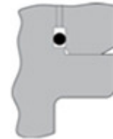
Fluoraz O-Ring Upper and Lower Body Seals in Stainless Steel Body Valves
