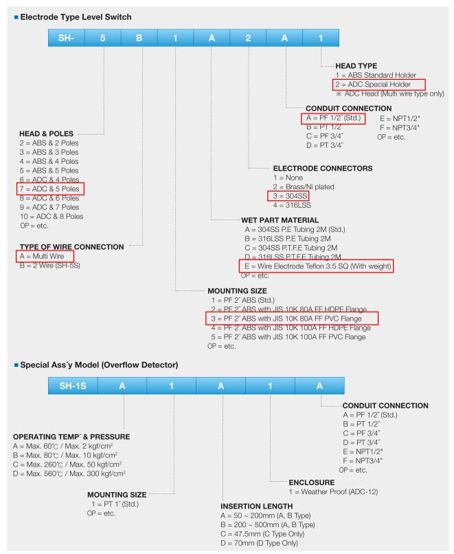
■ Special Ass'y Model: SH-1S (Applicable to over flow detection type)
