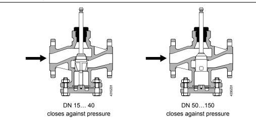
Guided plug which is integrated in the valve stem. The seat is machined in the valve body. Schematic representation, design variations are possible.
