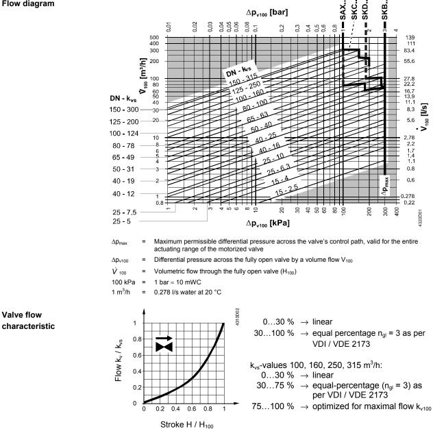
Cavitation accelerates wear on the valve plug and seat, and also results in undesirable noise. Cavitation can be avoided by not exceeding the differential pressure shown in the "Flow diagram" on page 5, and by adhering to the static pressures shown below.
