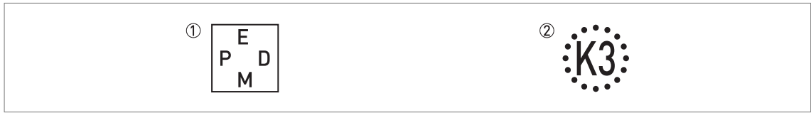
Figure 2-3: Symbols for the supplied gasket material (on the side of the process connection)
